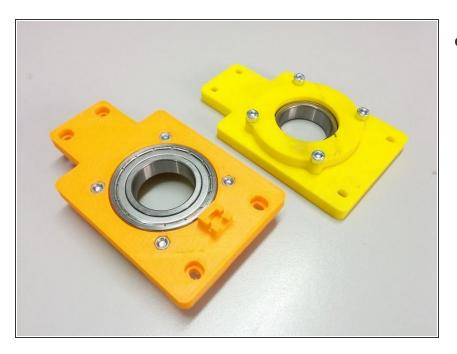
Finally, place the ball bearings inside the pockets created.
