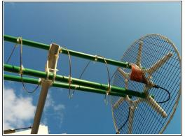
The 3 following pictures are from established RHCP antenna on the rotator. Polypropylene pipes were used instead of PVC. The total weight is 2.4 kg. Frequency 434 MHz
