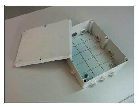
Start with your enclosure box. We are using an ABB 1SL0828A00 IP55 box.
